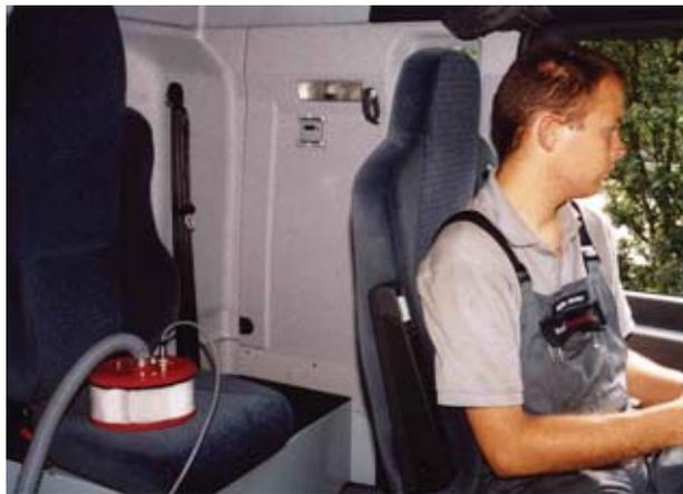
Fig. 11. Nanocleaner placed in a truck cabin. Two units are used for the test measurements
