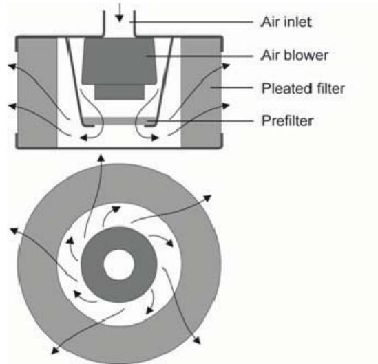
Fig. 3. Setup of the filter with integrated prefilter for coarse particles and blower
