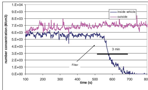
Fig. 8. Particle concentration inside and outside the car (passenger car). After turning the filter on, the inside concentration drops to very low levels over about three minutes
