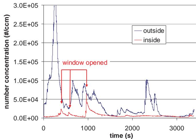
Fig. 14. Particle concentration inside and outside a coach. Three times, indicated by the red arrows, a window has been opened. Immediately the indoor concentration rises to approach the outdoor concentration and decreases again after the window is closed
