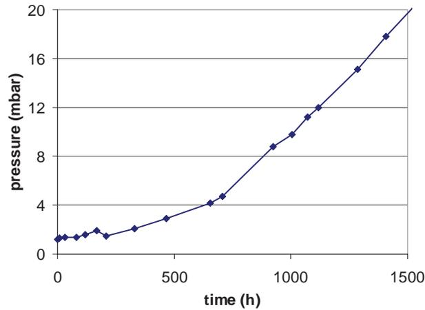
Fig. 5. Filter pressure drop as function of operating time in a highly polluted road tunnel
