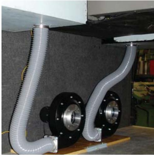
Fig. 13. Filter system for buses, installed in the luggage compartment
