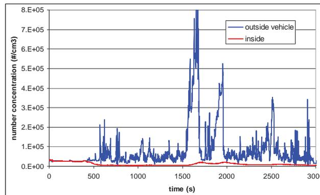
Fig. 9. Particle concentration inside and outside a passenger car with the filter turned on. Even when the external concentration is extremely high, in this example while driving through a tunnel, the indoor concentration remains very low
