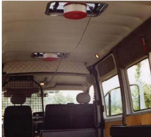
Fig. 10. Two Nanocleaner filter systems, mounted in a school bus
