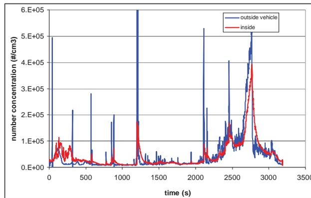
Fig. 1. Number concentration of particles inside and outside a car
