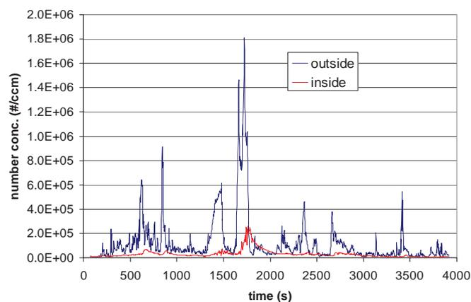
Fig. 12. Particle concentration inside and outside of the truck cabin
