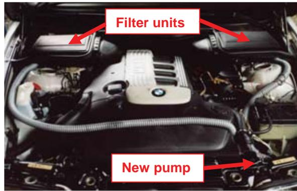
Fig. 15. The original filter of a BMW 530 has been replaced by high efficiency filters. Air is supplied by a blower which is also placed in the engine compartment
