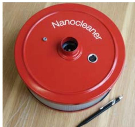
Fig. 4. Prototype of the filter system. Main filter, prefilter and blower are included. The system is operated by an external control box, containing the drive electronics for the blower and displays for filter pressure drop and time meter
