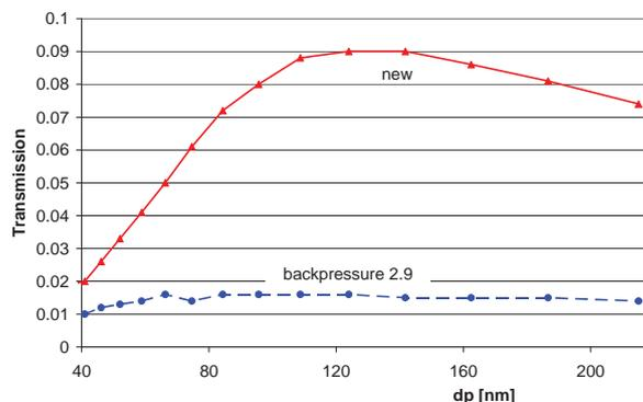
Fig. 2. Filter-efficiency: Transmission as function of particle size for the new filter and for the filter loaded to a pressure drop of 2.9 mbar
